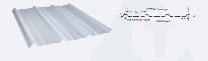
A PBR Panel is an 'R' style panel ideal for commercial roofing applications. It can be installed directly over purlins and joists because of it's Purlin Bearing Rib feature. This also creates an optimal seal for weather tightness, protecting your home from harsh weather conditions.
