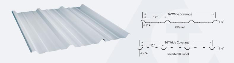
R Panel is a perfect fit for roofing and siding applications. The panels, commonly used in commercial applications, are lightweight and strong, allowing for easy installation and increasing the lifetime of your roof. An R Panel system from TCM gives you the flexibility to achieve the look you want with the advantages of metal roofing.
